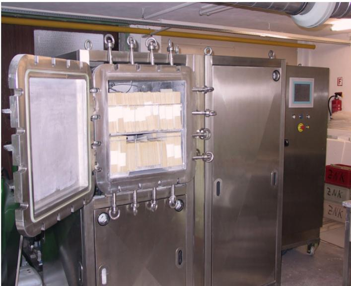
In the second half of the year under report, a newly designed - mobile - machine was installed at the ITS and the deacidification work was started.
